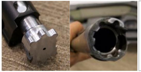
Unlike most shotguns, lock attaches directly to barrel itself from 6 lugs. This feature gives bigger and safer locking surface and easy opening of the lock with 15<sup>0</sup>'s turn.
