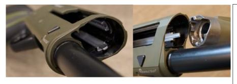
Stainless steel bolt moves in two steel rails attached to receiver, this way hardened steel bolt isn't wearing out the aluminum receiver and works with less friction thanks to surface quality of the rails. Male jut of the rail on the side slips into female gap in barrel extension and Male jut of barrel extension slips into female gap of the receiver.
