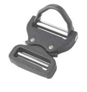
NEW ANSI rated COBRAFRAME MODELS Deluxe aluminium buckle with stainless steel adjuster bar, as 18 kN ANSI rated version. Belt width of 25, 38 and 45 mm are both available as standard and stretch version.
