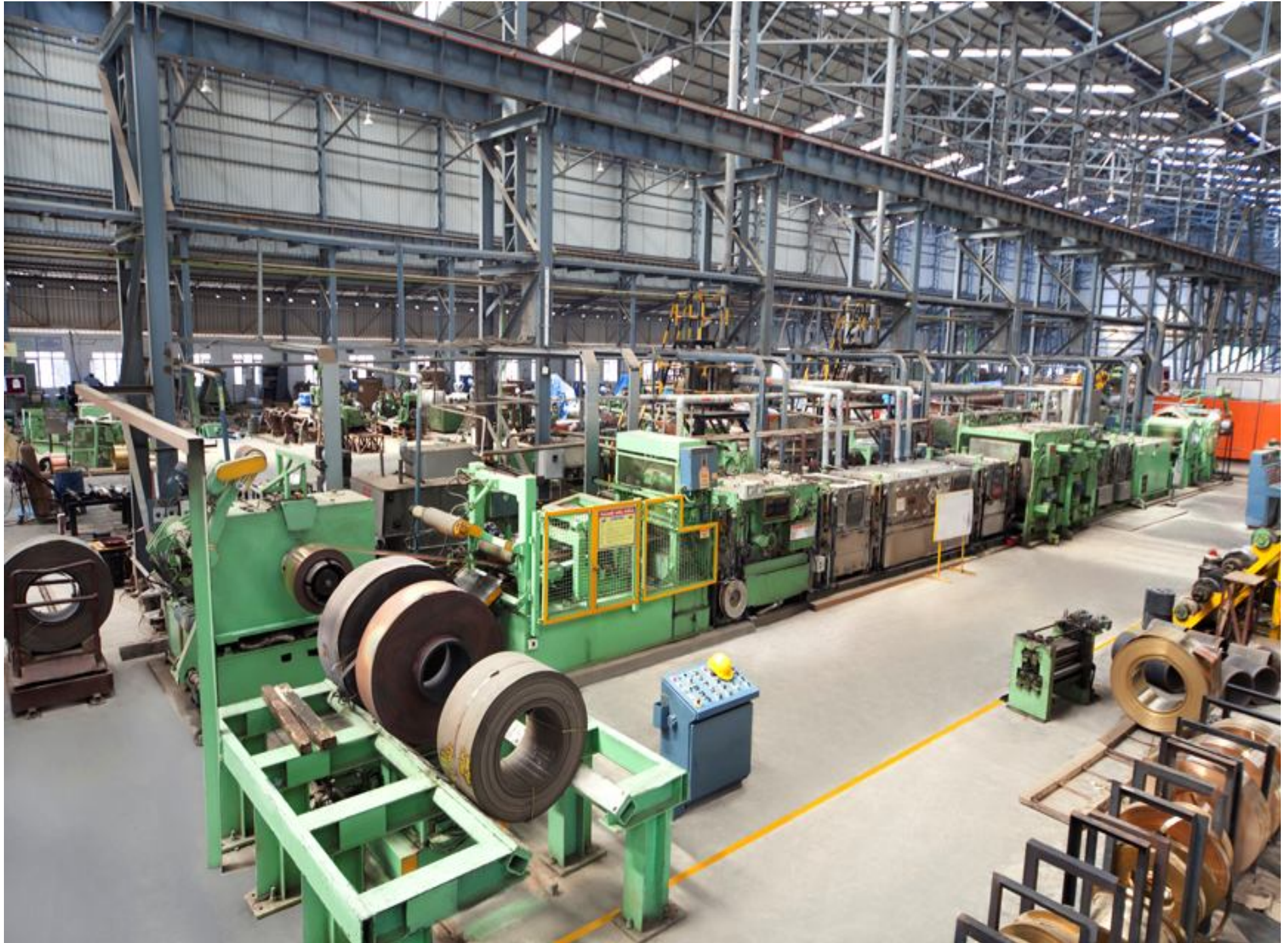
Pickling Line - Make: Wasero, Germany
