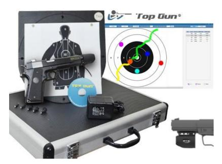
Users dry fire at an electronic target base, and important data such as: Statistical distribution of Hit Points, Aiming Path, Triggering Pull Movement, Aiming stability and habitual sighting error, are immediately displayed on their computers.
